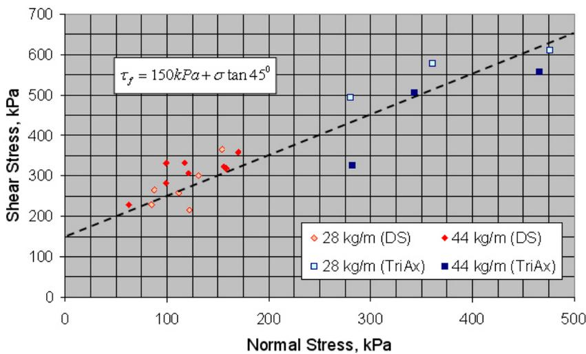
Figure 23. Shear strength of samples from LC columns determined by triaxial and direct shear tests.
