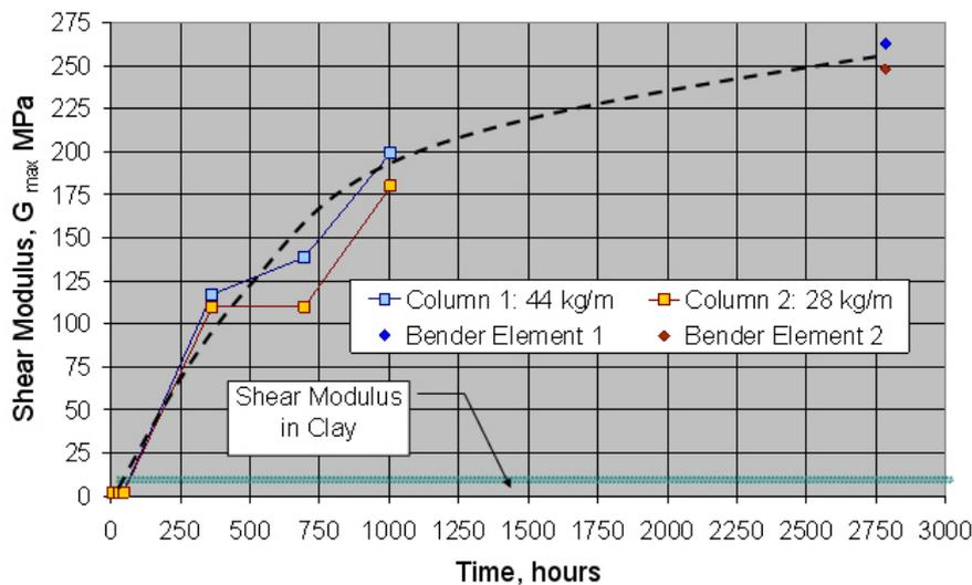
Figure 19. Variation of shear modulus  $G_{max}$  with time after installation of LC columns, cf. Figure 18.
