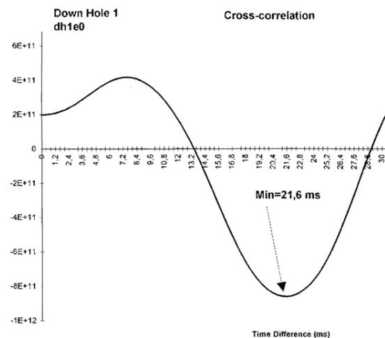
Figure 5. Determination of travel time between sensors using the cross-correlation method.
