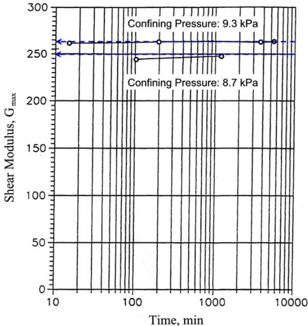
Figure 17. Results from bender element tests on consolidating sample from LC column.
