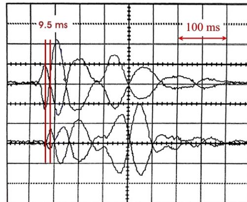
Figure 15. Signal from reverse impact test (depth interval 2.5 to 5.5 m) in column with mixing quantity 44 kg/m (156 kg/m<sup>3</sup>), 41 days after installation.
