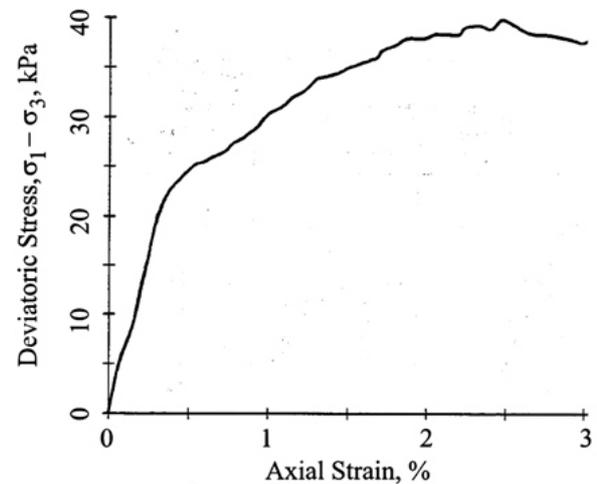
Figure 11. Triaxial undrained shear test on clay.
