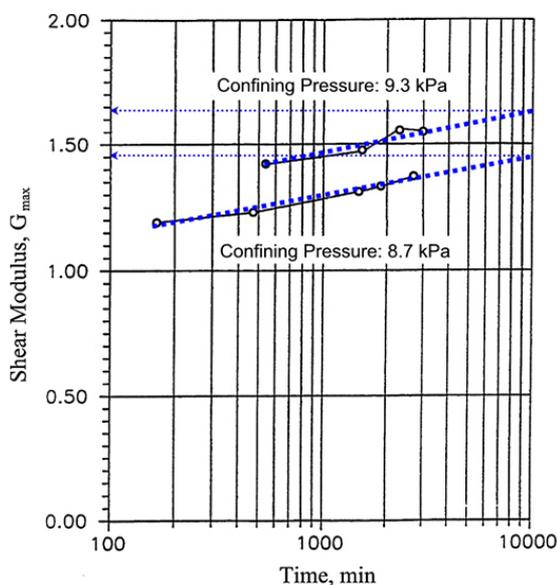
Figure 14. Shear modulus determined on clay sample from 3 m depth during consolidation at two different confining stresses.
