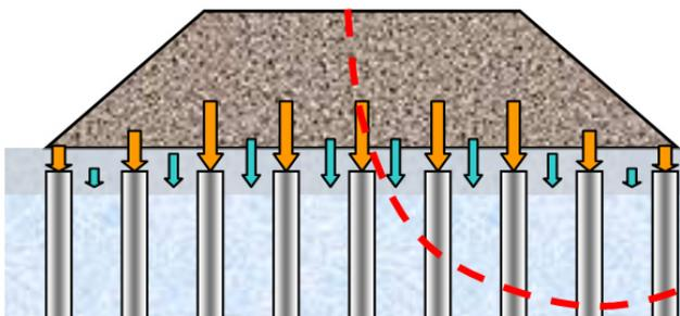
Figure 1. Load transfer from embankment to soil stabilized by columns.
