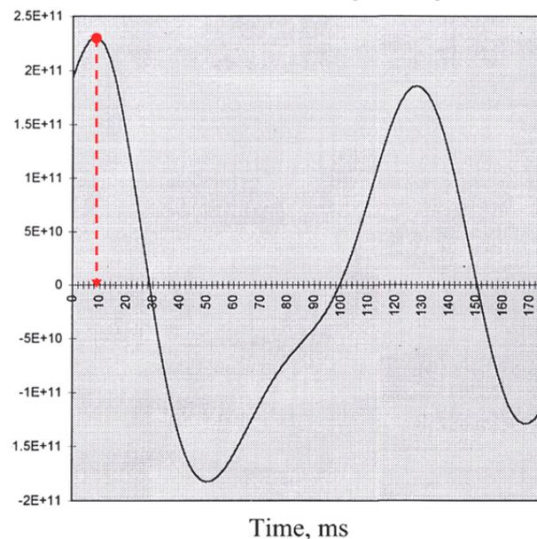
Figure 16. Determination of the shear wave velocity by cross-correlation of the signals shown in Figure 15.
