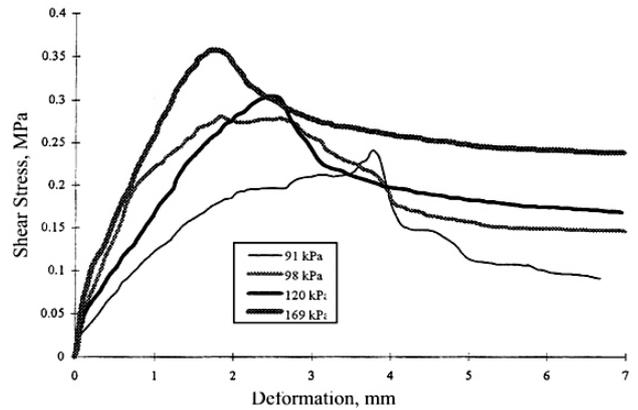
b) Mixing quantity: 44 kg/m (156 kg/m<sup>3</sup>)
