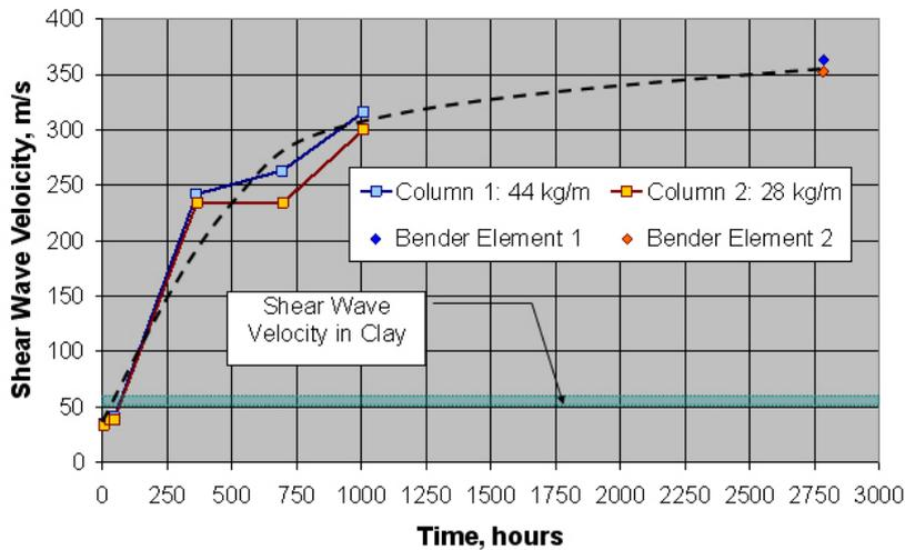
Figure 18. Variation of shear wave velocity with time, determined in-situ by down-hole tests and in the laboratory by bender element tests.
