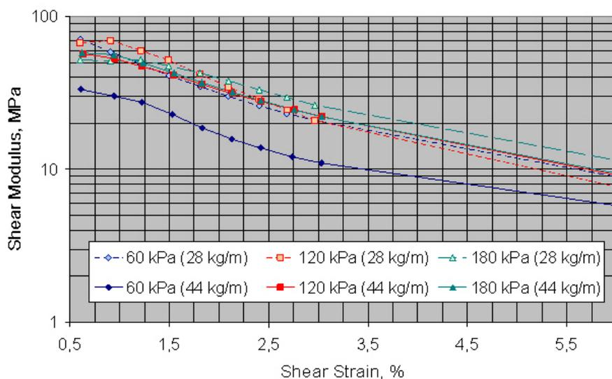
Figure 20. Shear modulus determined from triaxial tests within shear strain range of 0.5 to 6 %.
