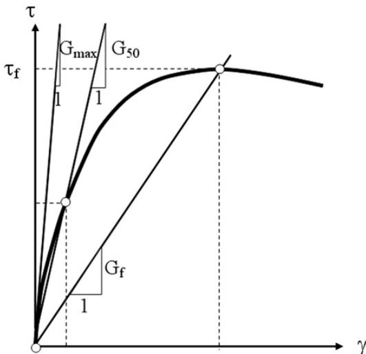
Figure 6. Shear stress – shear strain relationship for fine-grained soil at undrained loading.
