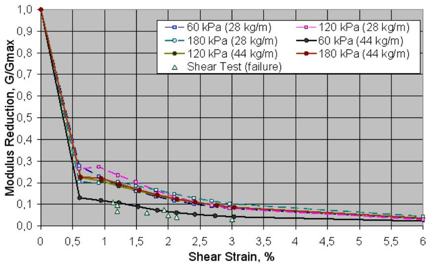
Figure 21 Decrease of shear modulus with shear strain for triaxial and direct shear tests.
