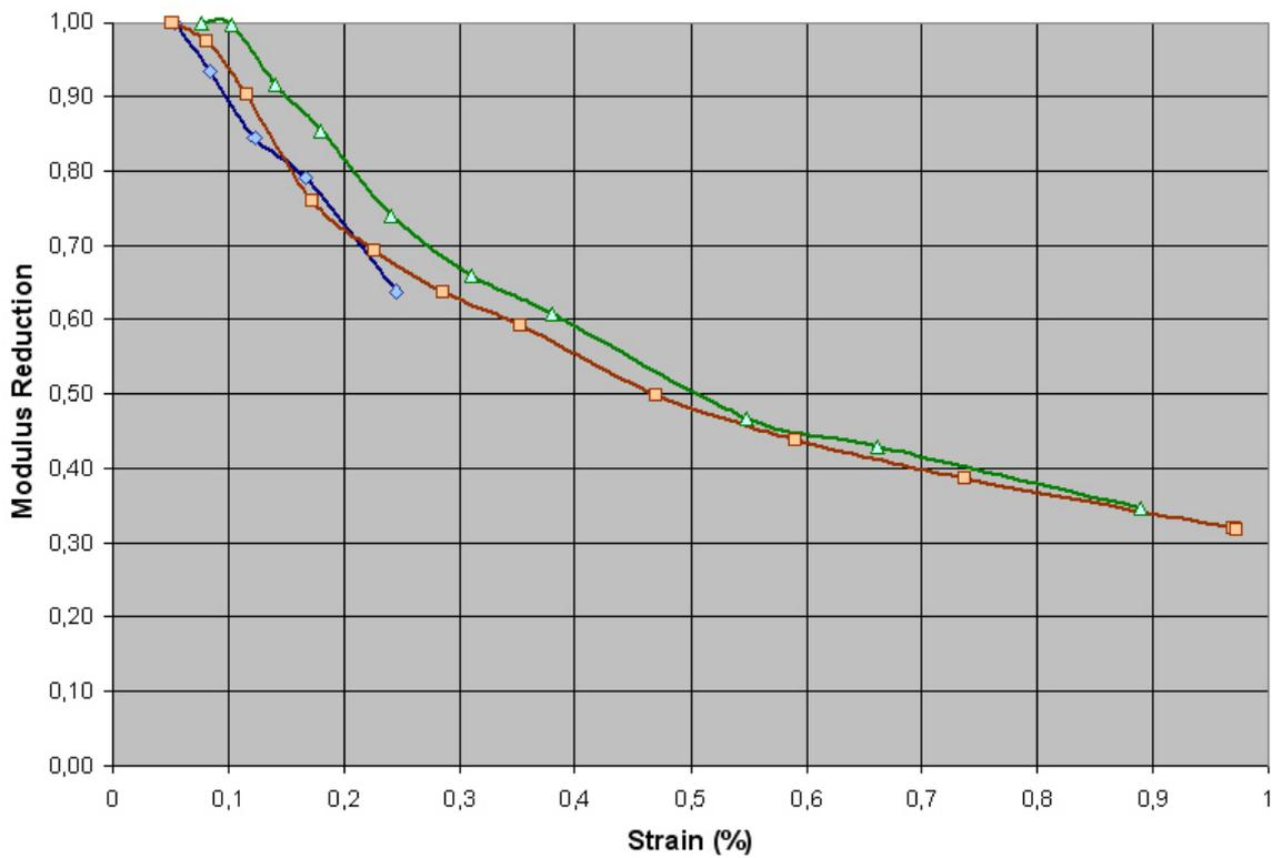
Figure 10. Reduction of compression modulus from field load tests on LC columns, after Kivelö (1994).
