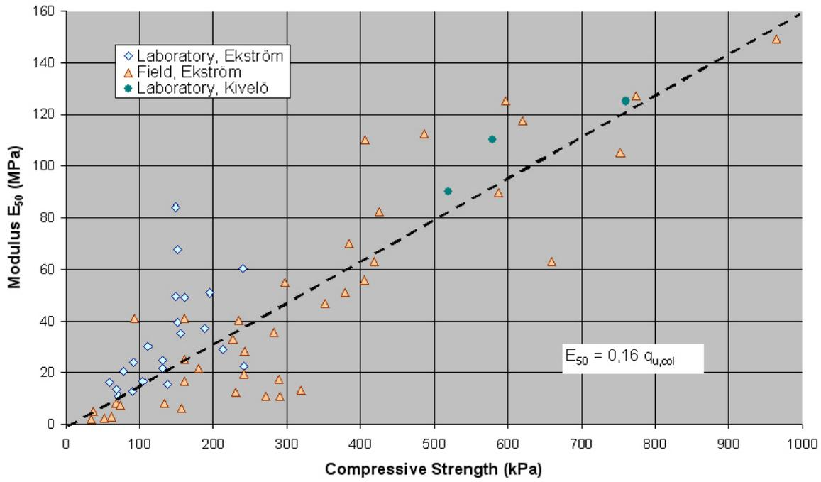
Figure 9. Relationship between the elastic modulus,  $E_{50}$  and the unconfined compressive strength from LC columns (Massarsch and Eriksson, 2002).
