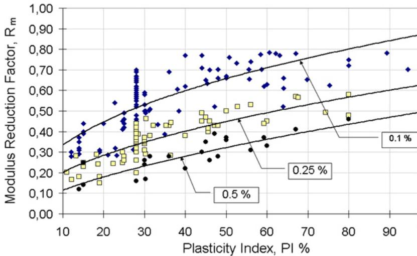
Figure 8. Modulus reduction factor,  $R_m = G_s/G_{max}$  as function of the plasticity index,  $PI$  at three strain levels, (Massarsch, 2004).
