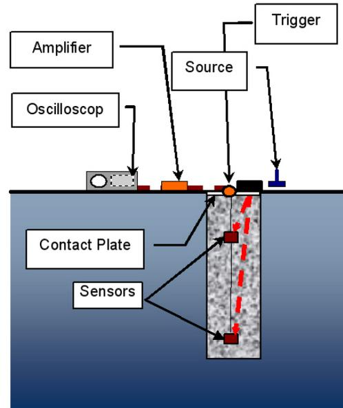
Figure 2. Principle of seismic down-hole test in LC column.
