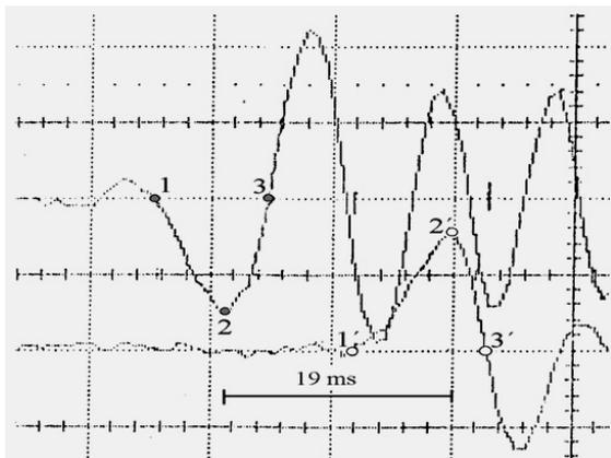
Figure 3. Determination of the first arrival time at different time intervals.
