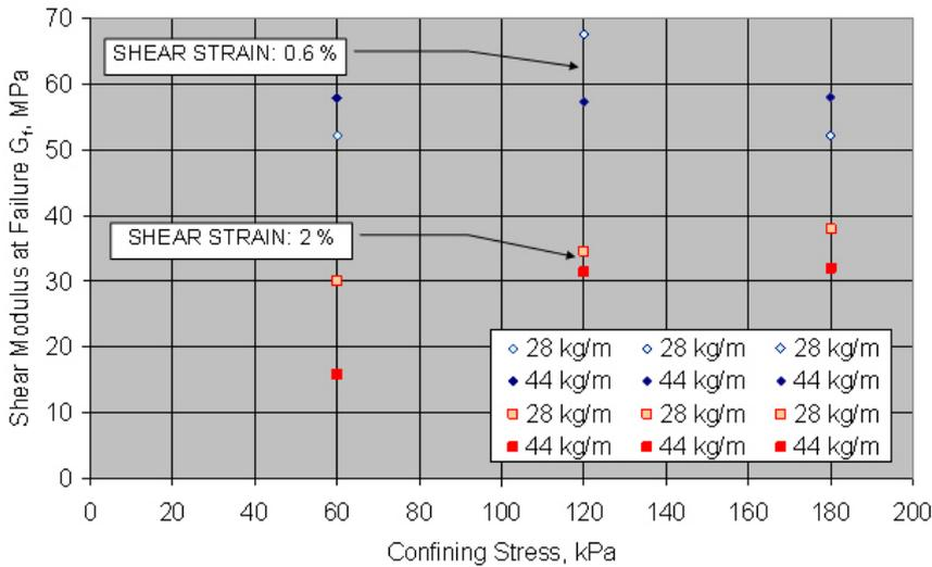
Figure 22. Variation of shear modulus  $G_{max}$  with confining stress at 0.6 and 2.0 % shear strain for columns with different mixing quantities.
