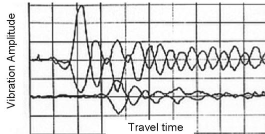
Figure 4. Reverse impact test of seismic down-hole test for determination of first arrival time.
