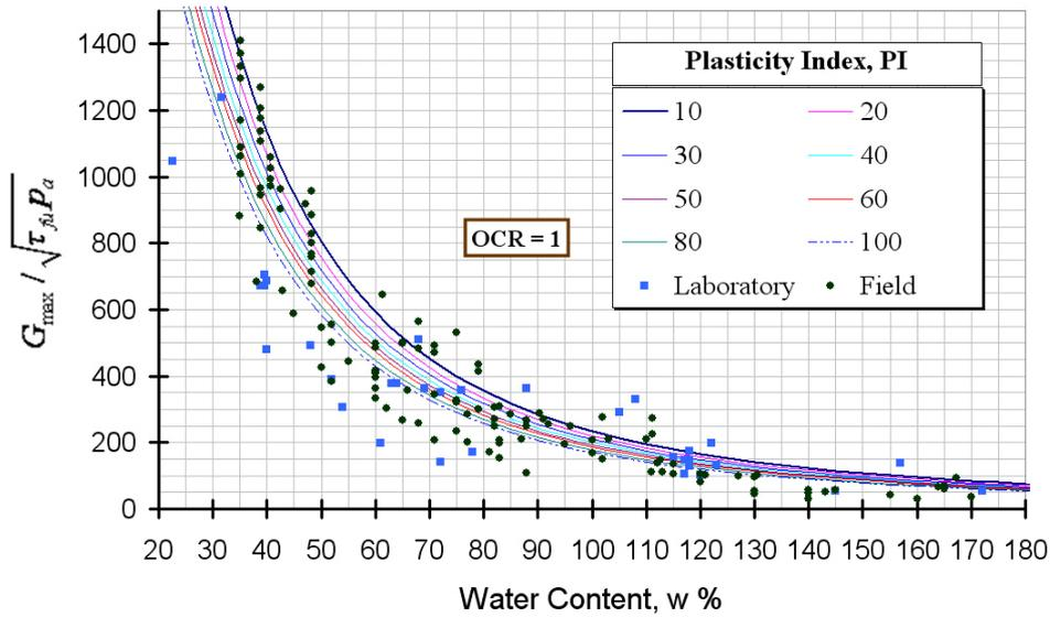
Figure 7. Relationship between the normalized shear modulus at small strains,  $G_{max}$  and the water content, cf. Eq.7; field and laboratory data from Döringer (1997).
