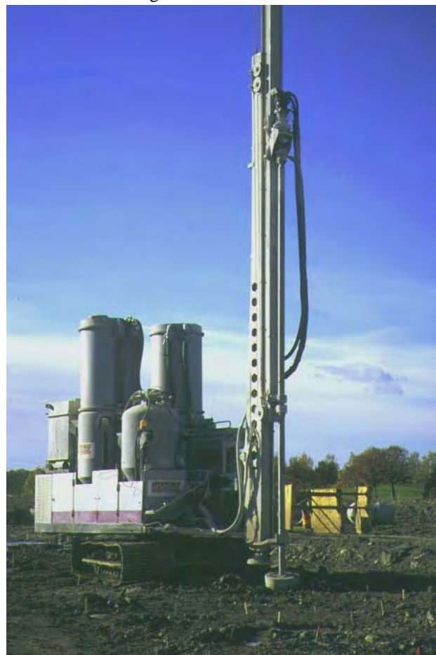
Fig. 9. Deep dry mixing equipment, mixing tool and base machine with containers for supply of binder (cement and lime).
