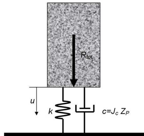
Figure 7. Model of pile base interaction according to Smith model.
