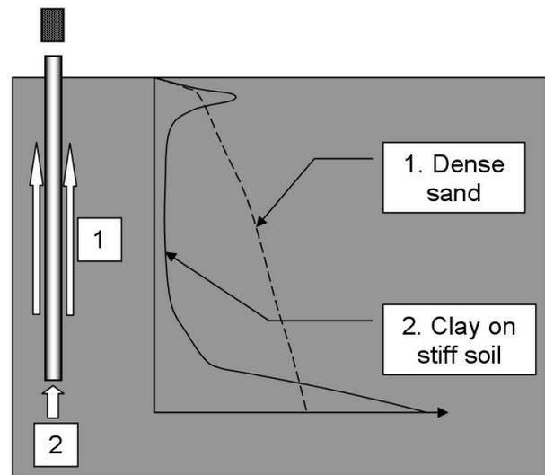
Figure 4. Conceptual picture of soil resistance along the shaft and base during driving of a pile into dense sand and soft clay on a stiff layer, respectively.
