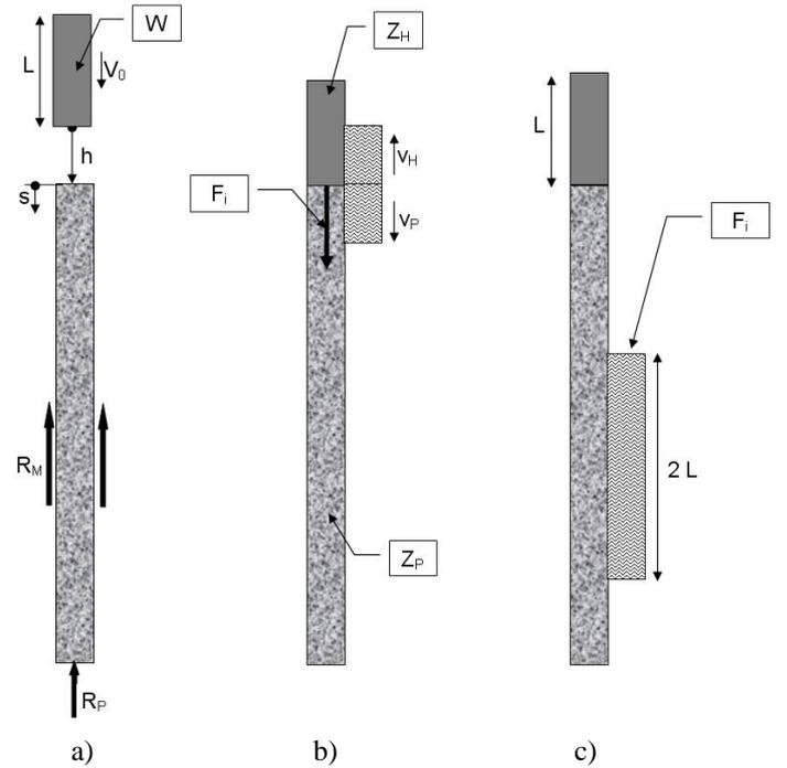
Figure 6. Definition of parameters governing stress wave propagation in piles.
