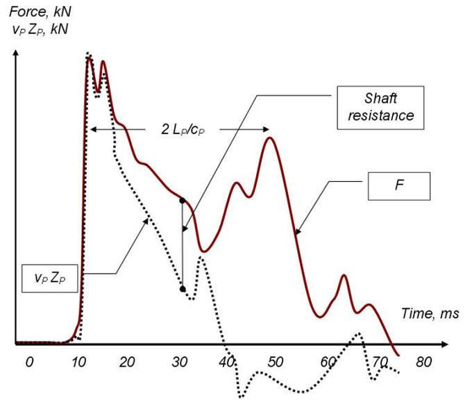
Figure 11. Principle sketch of results from stress wave measurements in a pile.
