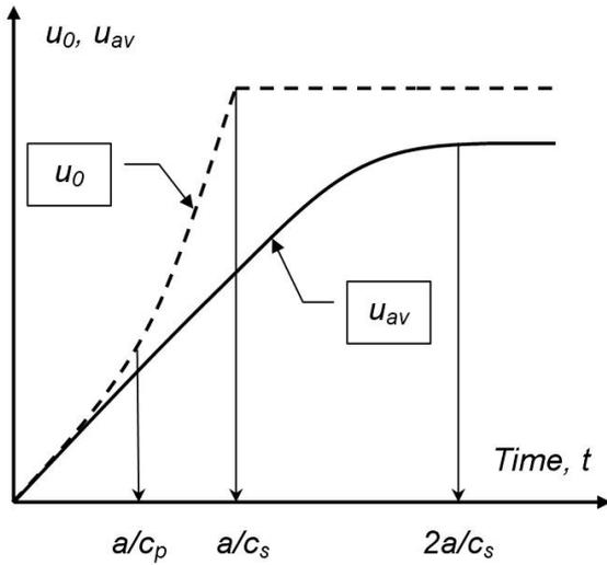
Figure 8. Schematic illustration of the displacement at the centre,  $u_0$  and the average displacement  $u_{av}$  due to a step load uniformly distributed across a circular area of radius  $a$ , Bodare & Orrje (1985), cf. equation (25).
