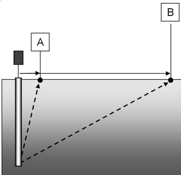
Figure 3. Influence of pile penetration depth on the distance to measuring points at two locations, A and B.
