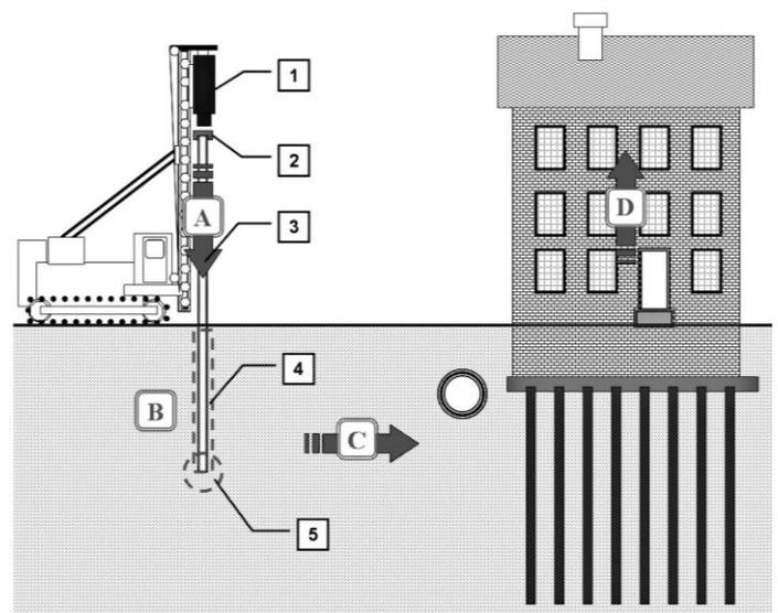
Figure 1. Transfer of pile driving energy from the hammer through the pile and into the surrounding soil and adjacent buildings.
