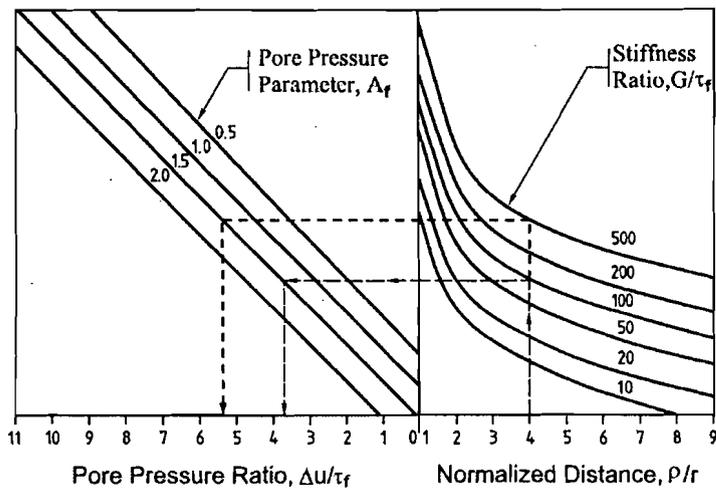
Fig. 8. Relationship between the excess pore water pressure in the vicinity of an expanding cavity for different stiffness ratios, MASSARSCH and BROMS [3]
