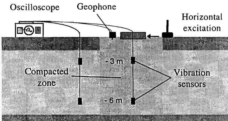
Fig. 9. Principle sketch of dynamic cross/down-hole test
