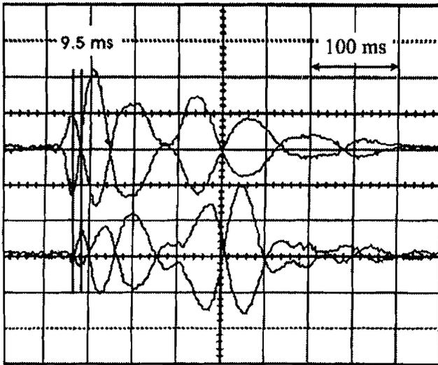
Fig. 5. Signal from reverse impact test (depth interval from 2.5 to 5.5 m) in column with a mixing quantity of 44 kg/m (156 kg/m<sup>3</sup>), 41 days after installation
