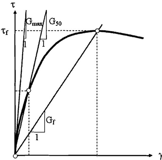
Fig. 1. Shear stress–shear strain relationship for fine-grained soil at undrained loading
