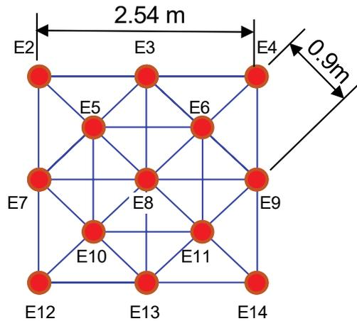
Fig. 6. B.E.S.T. Pile group configuration (E2 – E14).
