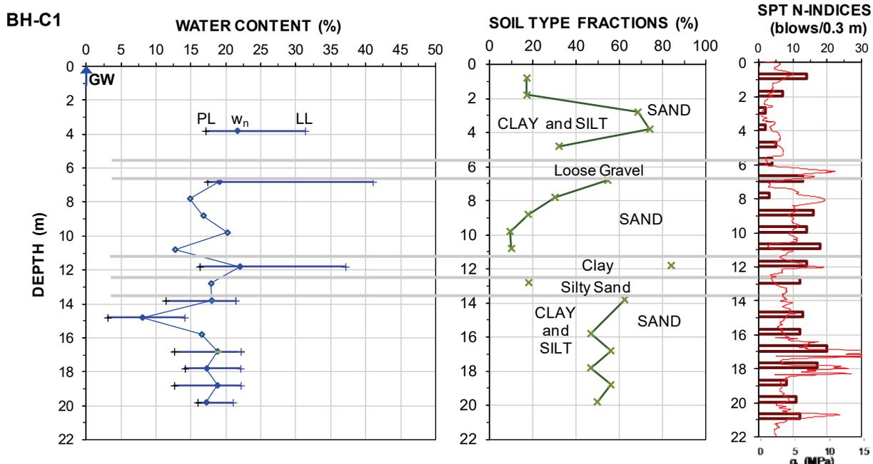
Fig. 10. Borehole data and SPT N-values, BH-C1.
