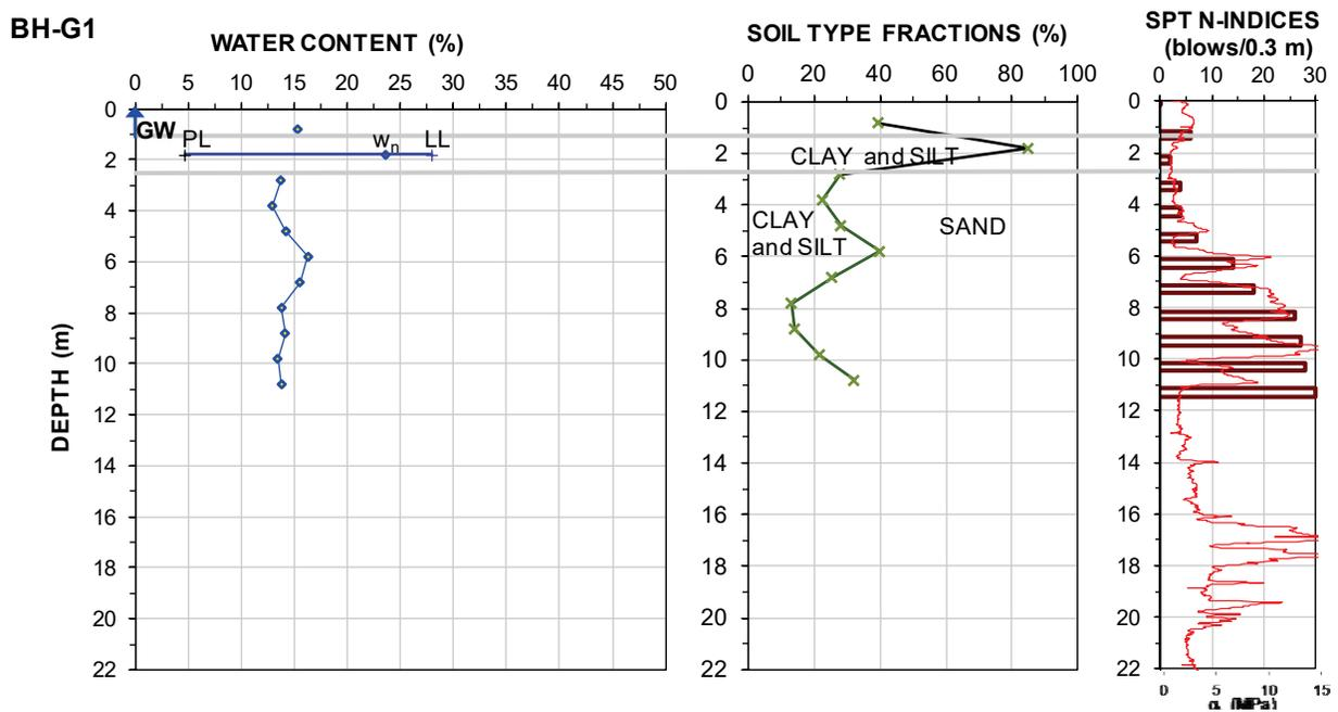
Fig. 15. Borehole data and SPT N-values, BH-G1.
