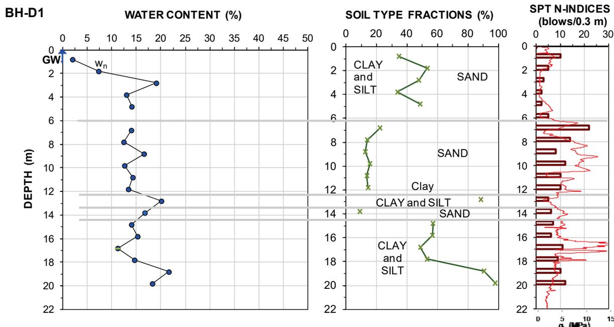
Fig. 11. Borehole data and SPT N-values, BH-D1.
