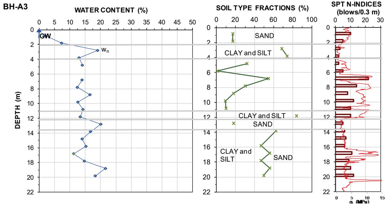
Fig. 8. Borehole data and SPT N-values, BH-A3.
