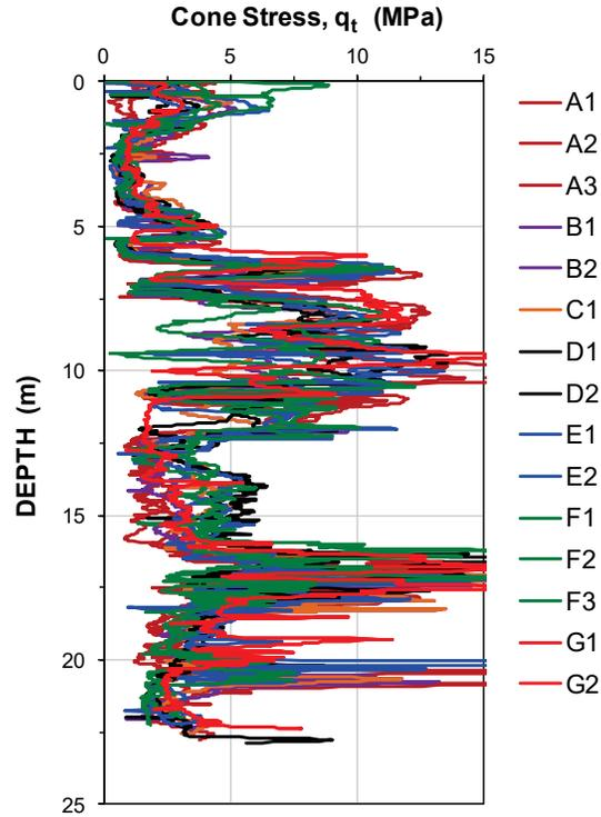
Fig. 16. CPT  $q_t$  records from 15 tests.
