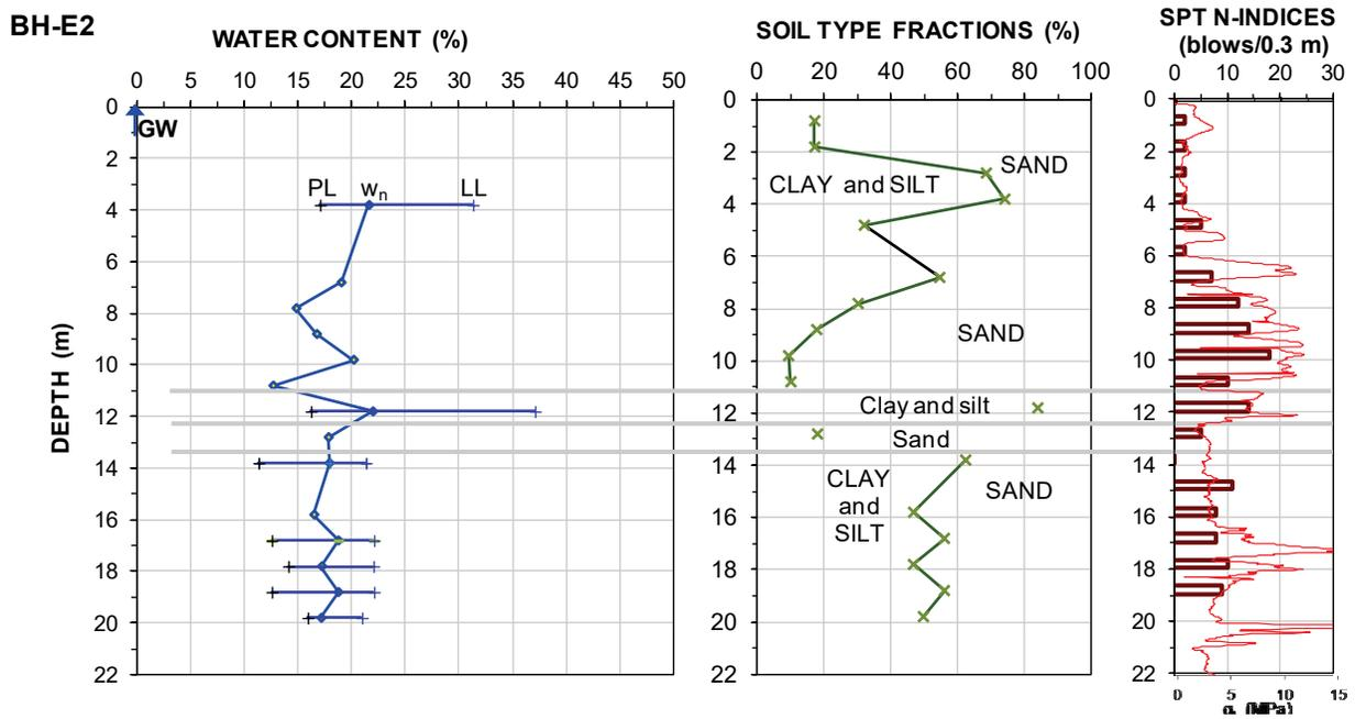
Fig. 13. Borehole data and SPT N-values, BH-E2.
