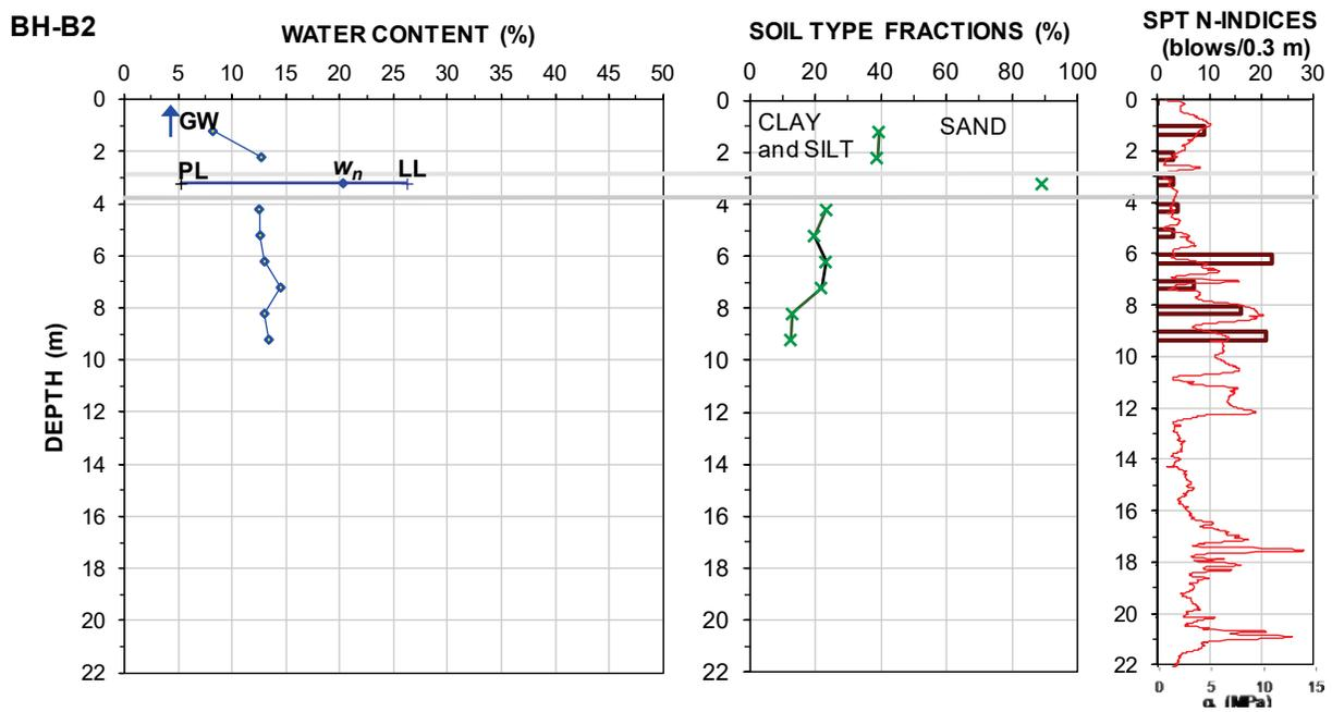
Fig. 9. Borehole data and SPT N-values, BH-B2.
