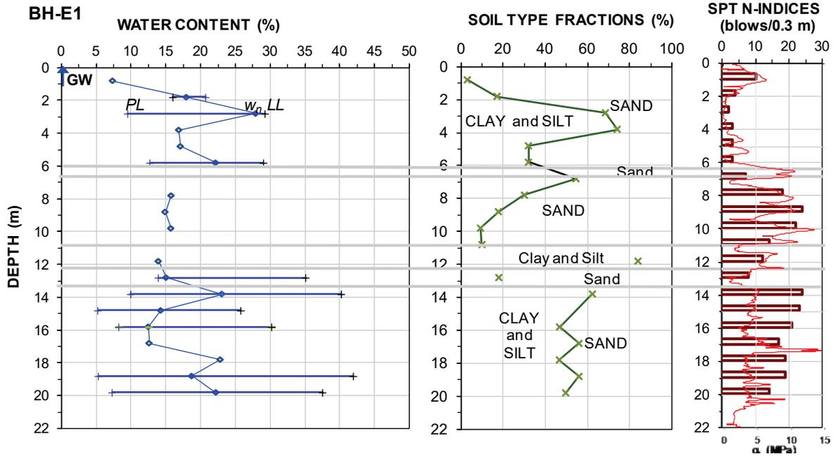
Fig. 12. Borehole data and SPT N-values, BH-E1.
