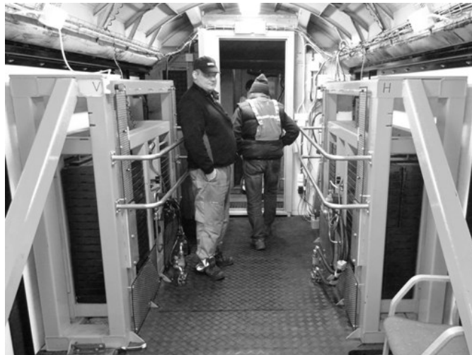
Fig. 1. View inside of the RSMV, showing oscillating masses on either side
