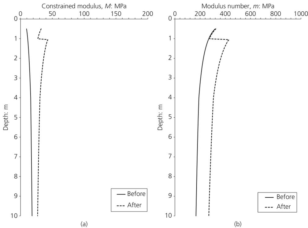
**Figure 6.** (a) Constrained modulus and (b) modulus number before and after compaction obtained with assumed CPT data (see Table 4). Note that the same scale was chosen as in Figure 4 to facilitate comparison of data
