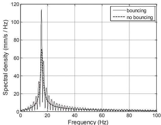
Figure 13. Influence of bouncing for a 100 kg hammer.
