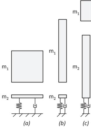
Figure 9. The three different SDOF models.
