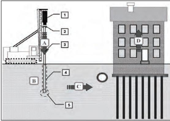
Figure 1. Process of energy transfer during pile driving, after Massarsch (2005).
