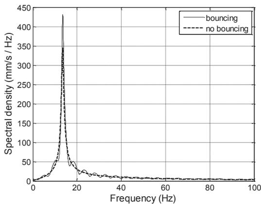
Figure 14. Influence of bouncing for a 500 kg hammer.
