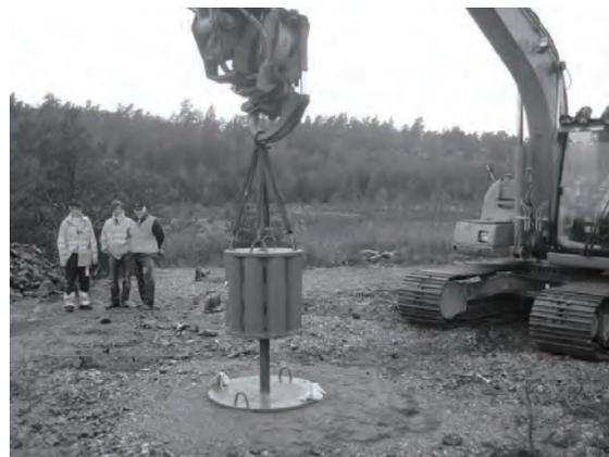
Figure 4. Falling weight tests.
