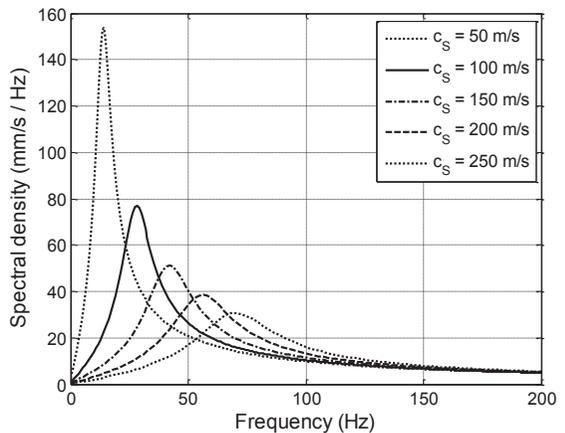
Figure 10. Calculated velocity spectrum with varying shear wave speed.
