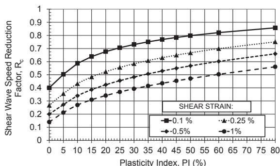
Figure 3. Reduction of  $c_s$  as a function of  $PI$  for cohesive soils for different shear strain levels, based on Massarsch (2004).
