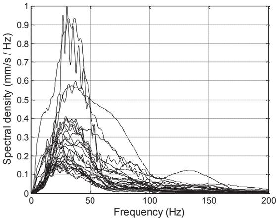
Figure 5. Average velocity spectra at all drop points.
