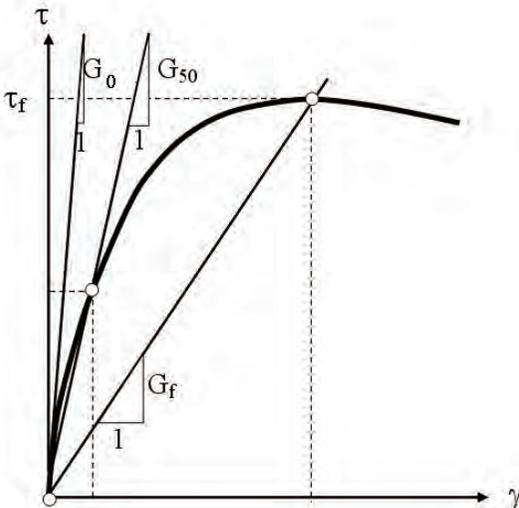
Figure 2. Shear stress-shear strain relationship for soil, after Massarsch (2004).
