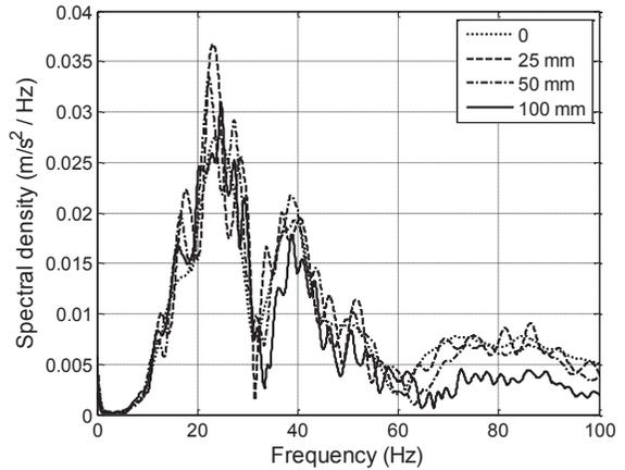
Figure 7. Influence of rubber pad thickness.
