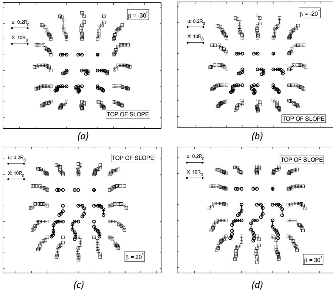
FIG 12. Effect slope inclination on lateral displacement of soil and piles.
