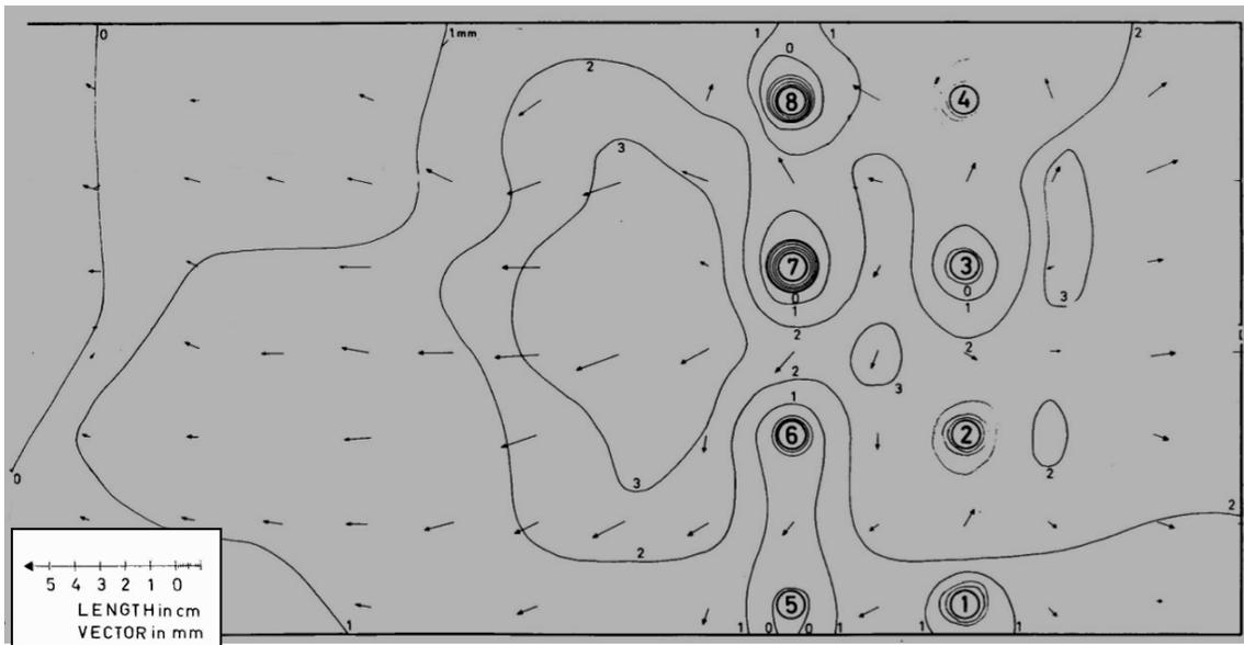
**FIG 5. Cumulative surface displacement after driving of two pile rows, showing lateral displacement vectors and heave of soil surface, cf. Figure 4.**
