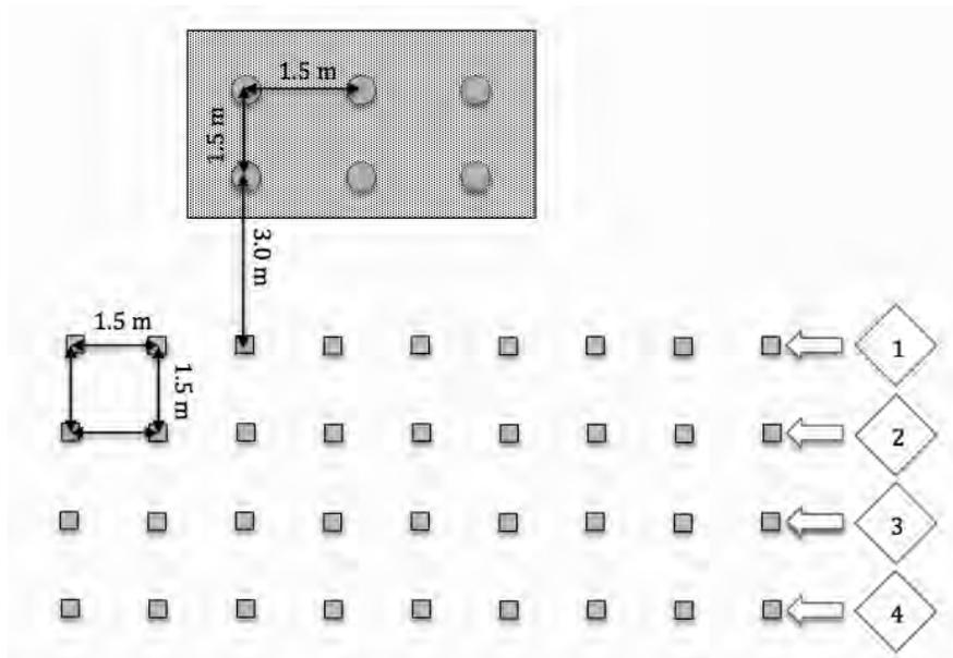
FIG 13. Pile group driven adjacent to an existing pile-supported bridge foundation. Sequence of driving pile rows and driving direction are indicated.
