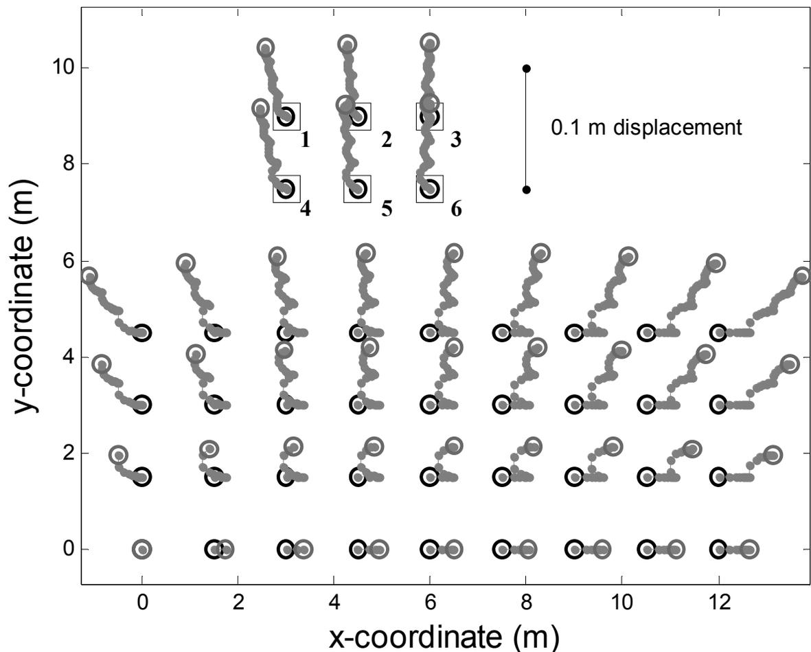
**FIG 14. Calculated lateral displacements of heads of driven piles and of existing piles of bridge foundation (refer to Table 1 for pile numbers). Black and red circles indicate the start and end point of the displacement path. Pile displacement 25 times magnified.**
