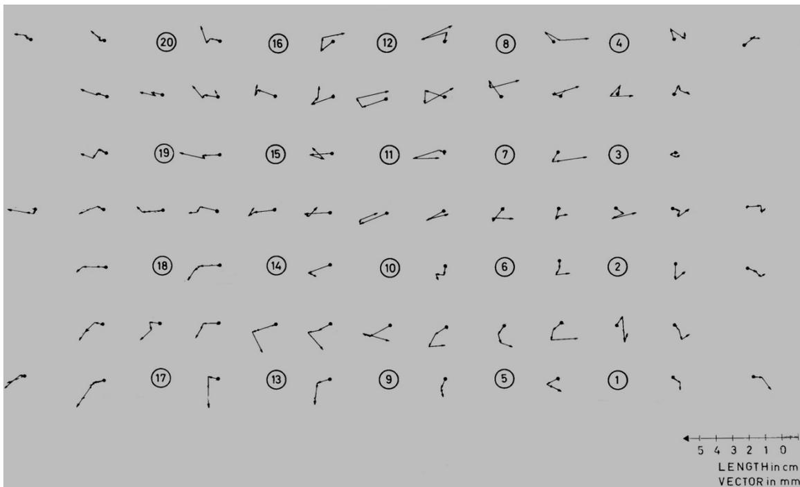
**FIG 6. Incremental surface displacements after driving of two, three and five pile rows.**
