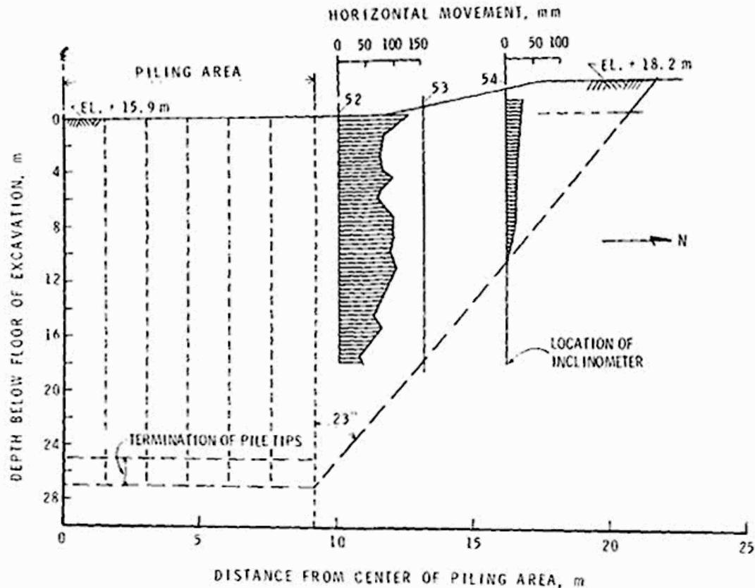
**FIG 9. Horizontal soil movements determined by inclinometers north of the piling area, Bozozuk et al. (1978).**
