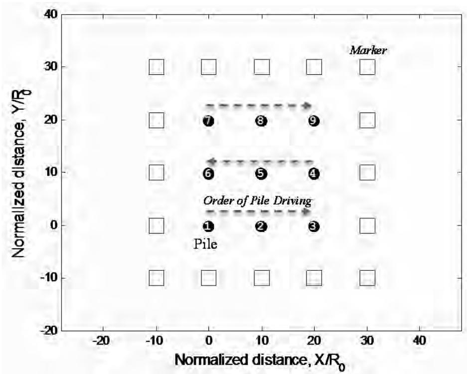
a) Geometric arrangement and sequence of pile driving
