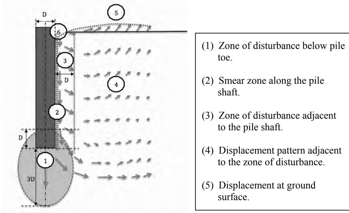
**FIG 1. Schematic illustration of the displacement field and zones of disturbance during pile installation.**
