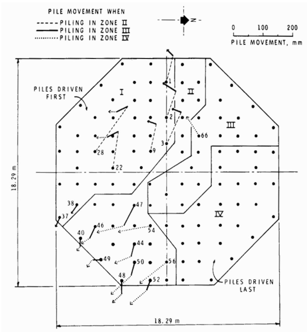
**FIG 8. Photographic measurements of horizontal pile movements due to pile driving, Bozozuk et al. (1978).**
