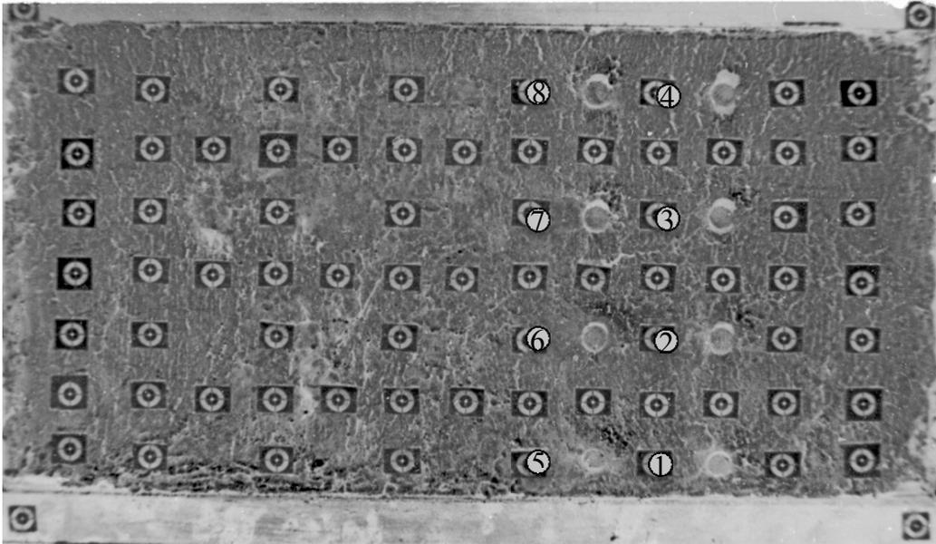
**FIG 4. Surface of model box filled with clay after installation of two pile rows (8 piles), showing measuring targets and order of pile installation.**
