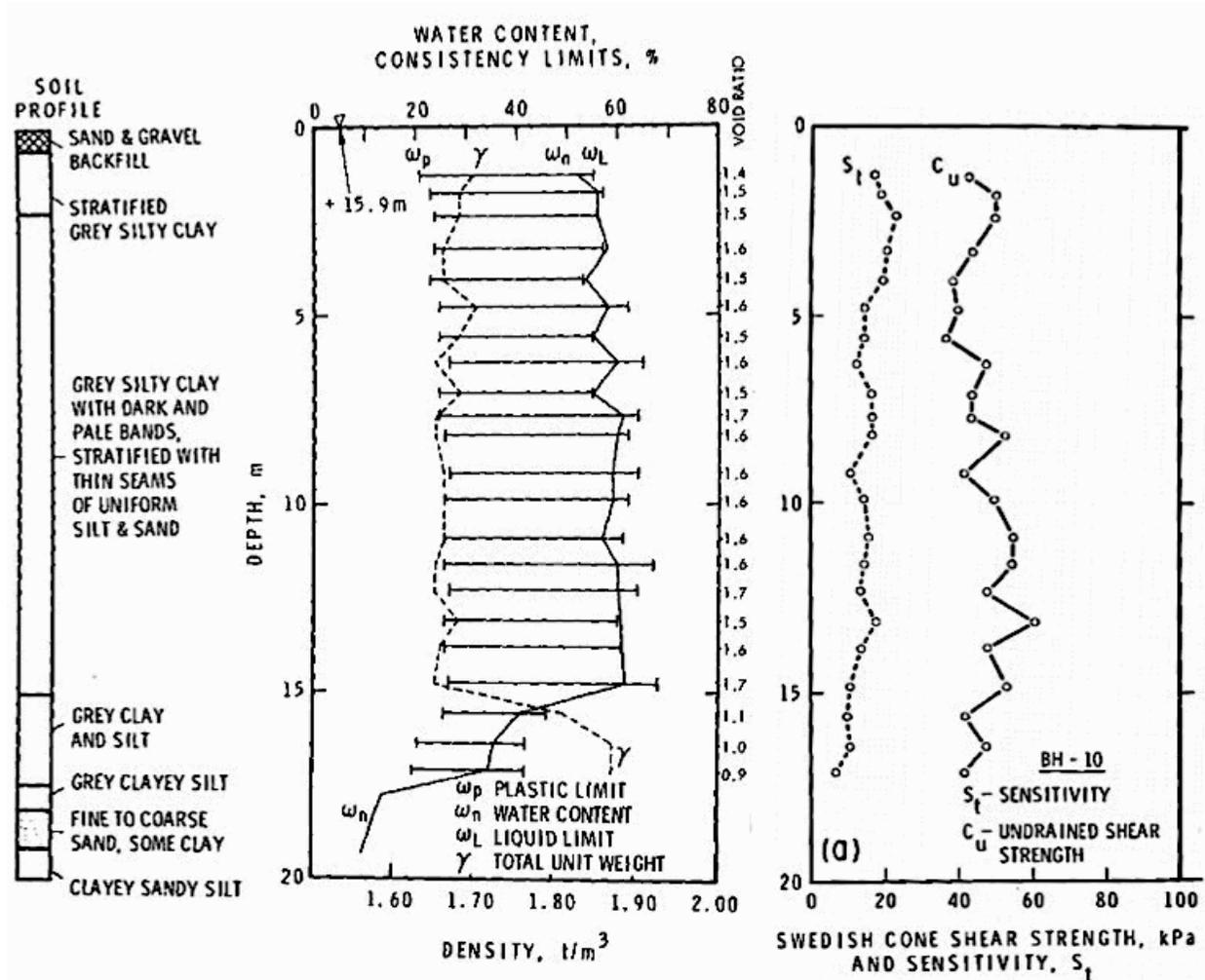
FIG 7. Geotechnical properties at piling site, from Bozozuk et al. (1978).
