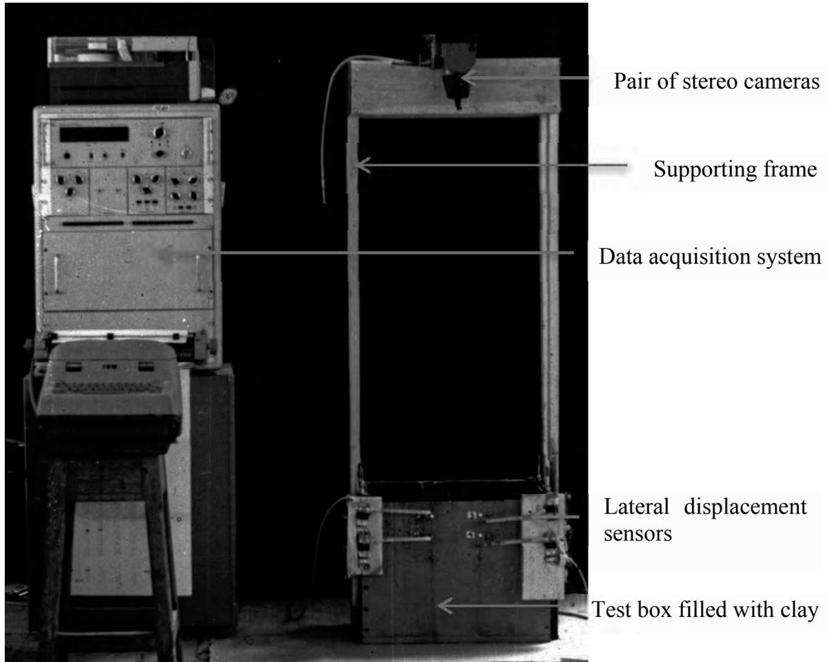
**FIG 3. Stereo-photogrammetric equipment for measurement of surface displacements.**
