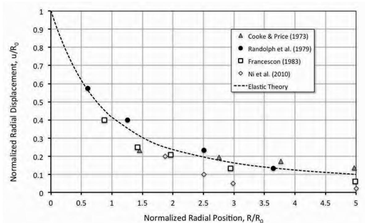
**FIG 2. Variation of radial soil displacement according to Eq. 1 and comparison with model tests reported in the literature.**
