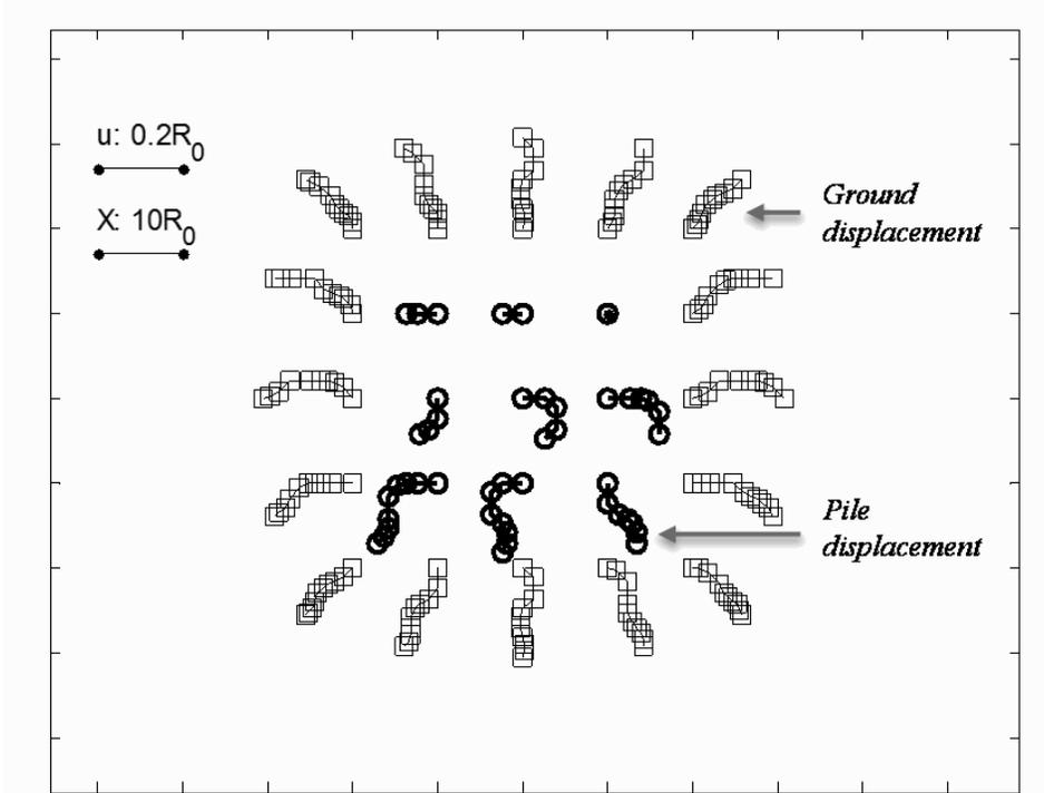
b) Lateral displacements due to driving of pile group
