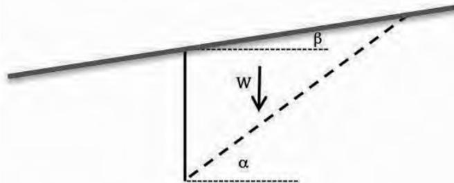
**FIG 11. Assumptions regarding the effect of inclined ground surface on expansion of cylindrical cavity.**
