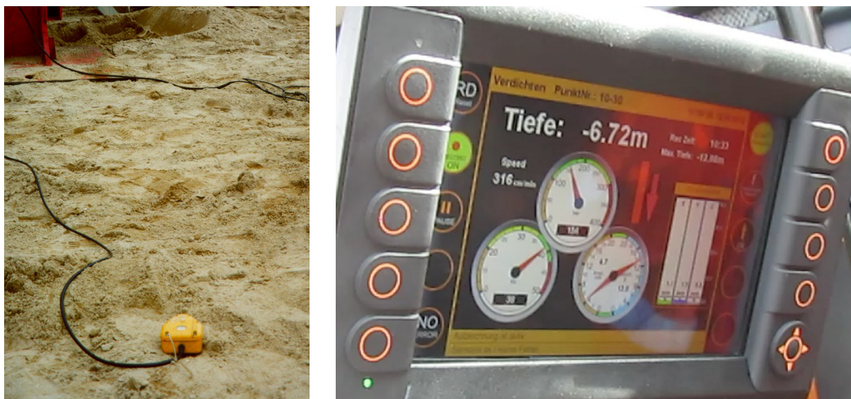
a) Ground vibration measurement by tri-axial geophone b) Display of vibration parameters measured during pile penetration (System Gamperl und Hatlapa)
