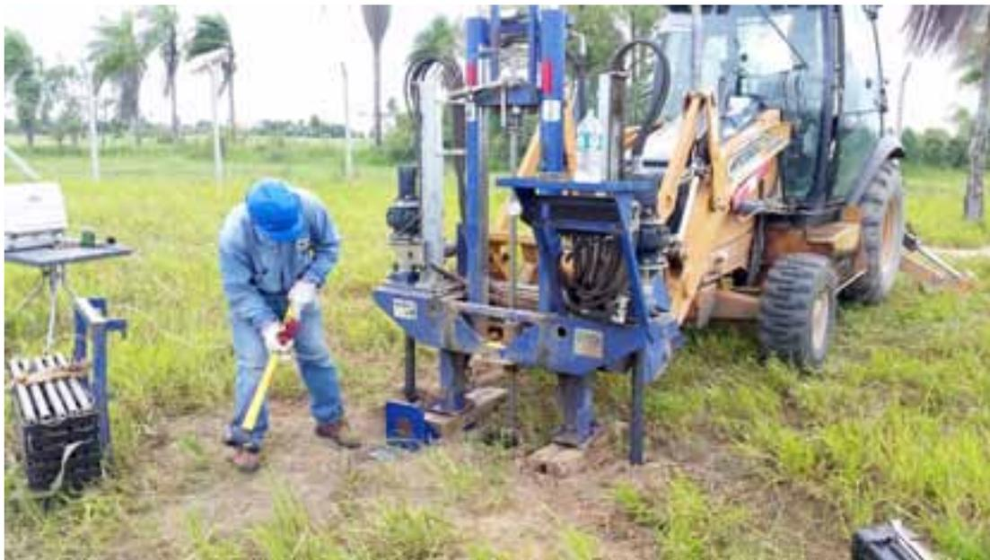
Fig. 8. Execution of a seismic down-hole test (SDMT) at the B.E.S.T. site, courtesy Incotec.
