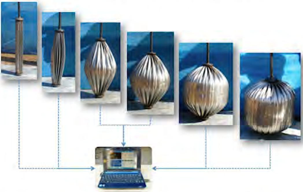
Fig. 1. Expansion steps of the EB Incotec (EBI) with field monitoring by data acquisition system.
