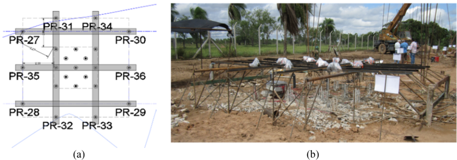
Figure 7. (a) General arrangement of at the test, showing reaction piles and beams; (b) Frame for recording pile movements Phase I test on Piles E2 - E14.
